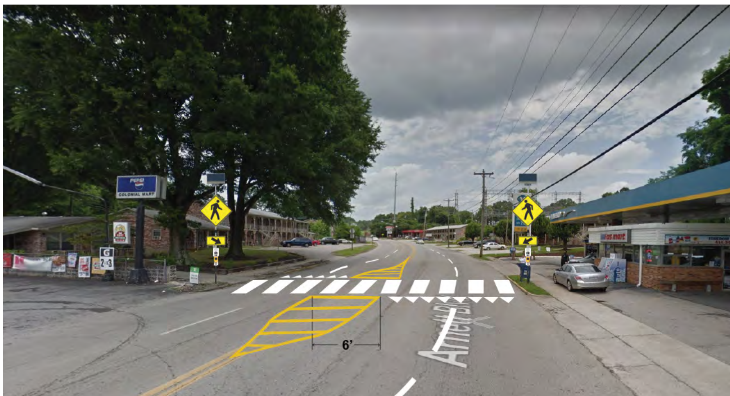
Figure 15b. Illustration of Proposed Crosswalk design with Pedestrian Refuge
